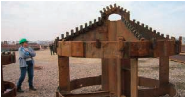
[Fig. 8] 2.5 m Dia. Drill Bit
