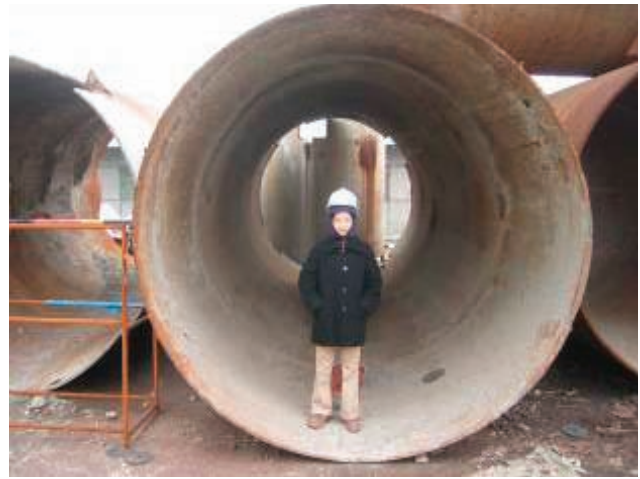
[Fig. 5] 2.8 m Dia. Drill Casing
